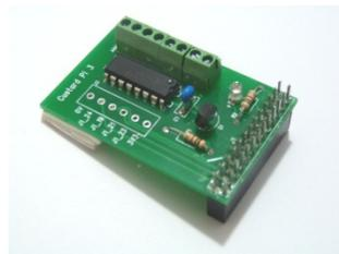
For ease of assembly, this project uses a Custard Pi base and a prototyping board. The assembled hardware is shown below.
