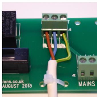
Once the product is assembled and shown to be working correctly, we recommend using hot melt glue where the cable enters the screw terminals to prevent strands of wires accidentally touching each other.
